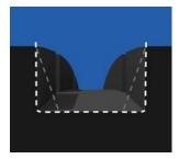
U SHAPE GROOVES Grooves "side walls" are more 'vertical', which increases void ratio at 2mm remaining tread depth & allows higher water evacuation.
