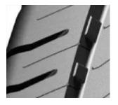
**STONE EJECTOR** Prevents stone retention, resulting in improved service life.
